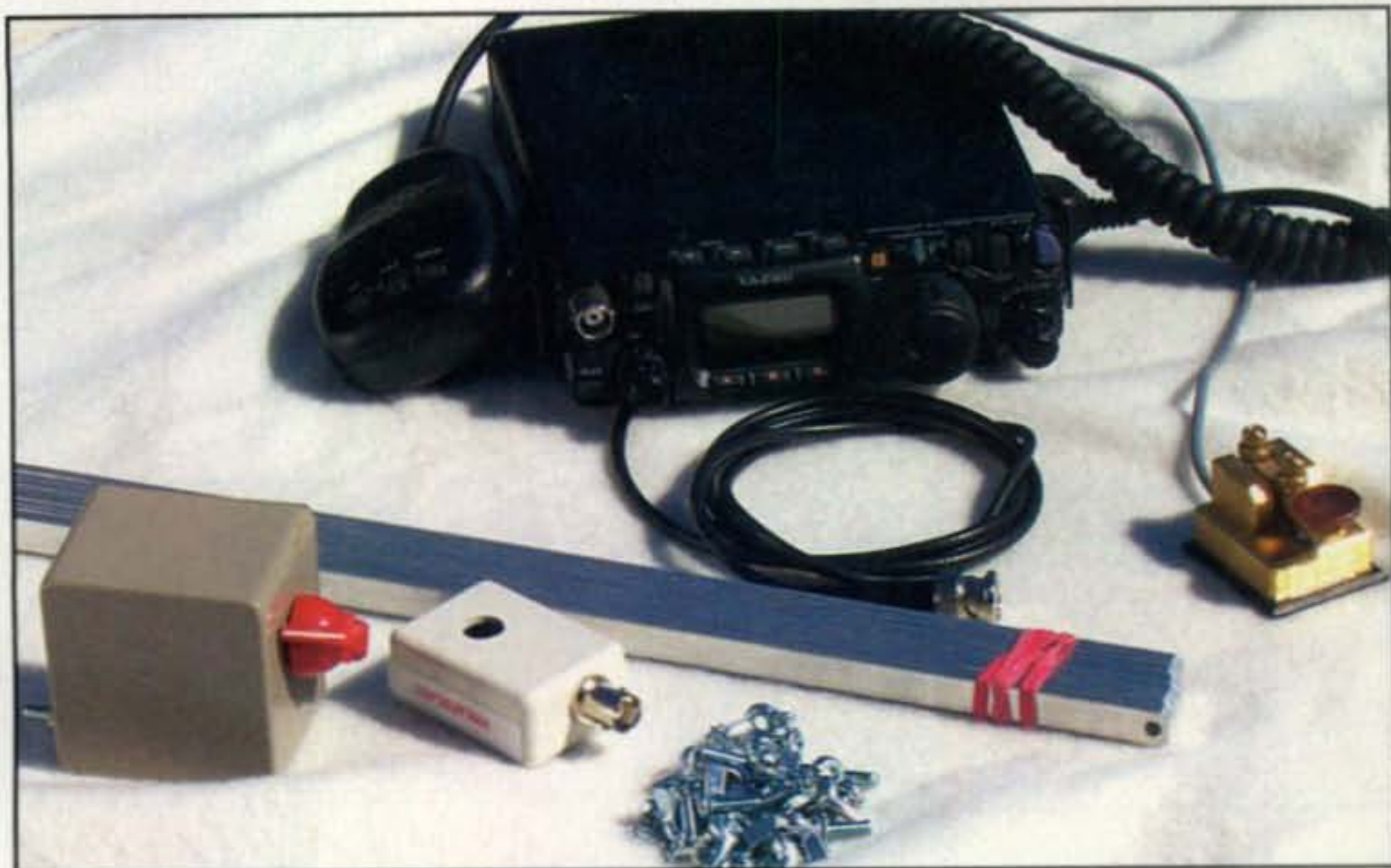
Photo A— Ready to go QRP on 40, 30, and 20 meters with G4TPH's collapsible loop antenna.
